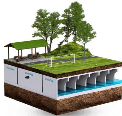
Figure 1-9. Subsurface storage system, generic example ( http://stormtrap.com/products/singletrap/ )
